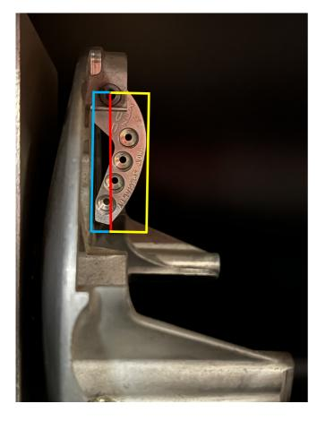
This cut-away of a Polaris clutch with Indy Specialty Clutch Master weights is to you understand the dynamics of our adjustable weights
