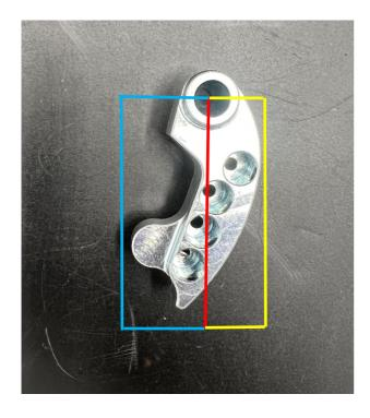
This cut-away of a Polaris clutch with Indy Specialty Clutch Master weights is to you understand the dynamics of our adjustable weights
